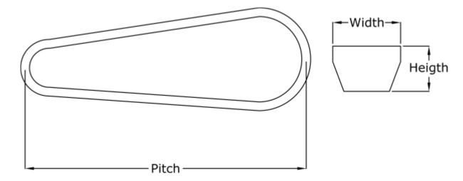
$\begin{array}{ll} \text{Datum Llength} = 2790 \\ \text{Height} &= 10 \\ \text{Length inside} &= 2770 \\ \text{Type} &= \text{BB107} \\ \text{Width} &= 17 \end{array}$
